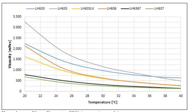
Measuring conditions: Rheometer, CP50-1, measuring gap 0.1mm
