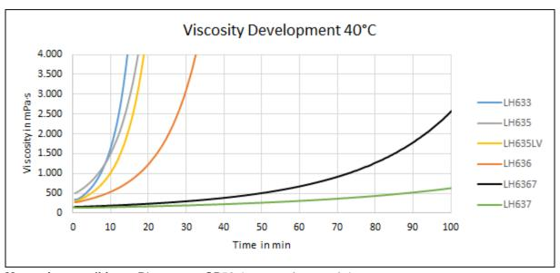
Measuring conditions: Rheometer, CP50-1, measuring gap 0.1mm
